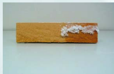
Dow Corning® MH-1109 Fluid protects against efflorescence in limestone.
